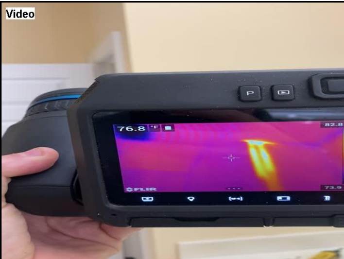
Video showing the area in the master bathroom where water is coming down inside the wall. This is below the shower upstairs.
